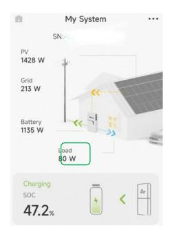
2). Operate the APP and follow the instructions below to enable function "Charge Batteries from Grid".
