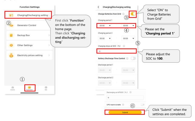
If the formula "Grid Power≈ **Load** + Battery Charging Power" fits well, the grid meter installation of the energy storage inverter is correct. Please remember to deactivate the "Charge Batteries from Grid" by clicking "OFF" and save the changes.
