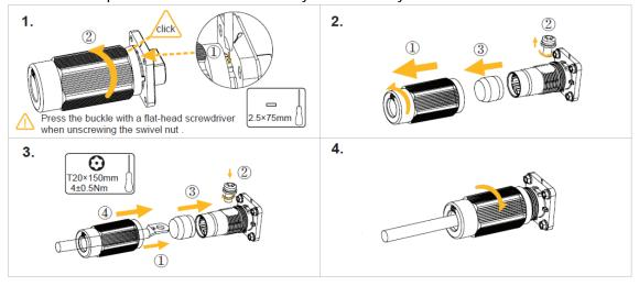
Press the buckle with a flat-head screwdriver (blade width: 2.5mm) when unscrewing the threaded sleeve of the battery power connector.
