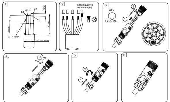
The steps for backup connection are similar to the grid connection, with a distinction in step 9:
