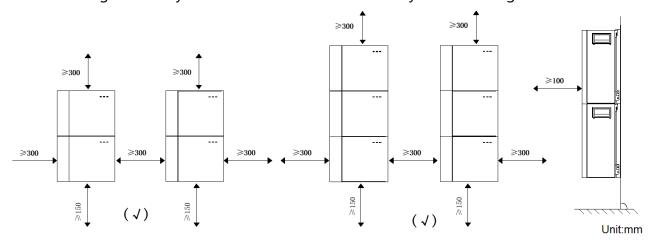
Local standards may add additional clearance requirements, particularly regarding clearances between the Battery System and other Electrical Appliances.
