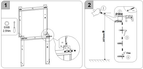
\* This recommended value "870mm" is for wall bracket location of the second battery seeing from the bottom up. This value may adjust depending on the number of expansion series batteries mounted later.
