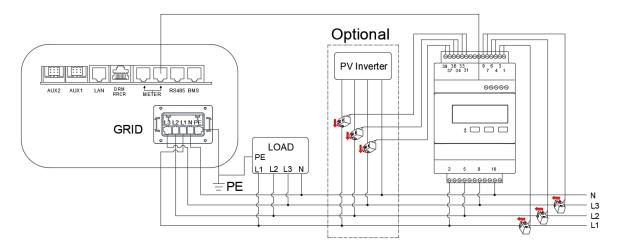
Meter communication cable requirements: standard network cable (recommended type: Cat5e, SFTP, UV-resistant for outdoor use).
