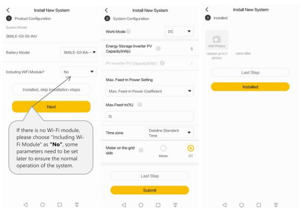
For regular installers, please click "Install New System", enter your installer account ID in the "license" field to bind the system to your account and "activate" the system. Enter S/N, check code, license, installation time and click the "save" button.
