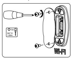
b. Tighten the Wi-Fi module onto the inverter with two M4\*12 screws provided (Tool: T20 screwdriver, torque: 1.6Nm). DO NOT OVERTIGHTEN – do not damage the plastic housing of the Wi-Fi module. Note that AlphaESS always recommends a LAN cable connection over the use of a Wi-Fi module.
