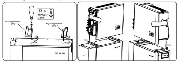
d. Attach the inverter to the side support feet. The inverter mounting holes should align to the horizontal holes of the side support feet. Note that the inverter sits inside (between) the two feet and is secured with two screws on the left and right sides.
