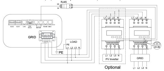
Meter communication cable requirements: two-core outdoor shielded twisted pair copper cable (flexible), conductor cross-section 0.5~1.5mm<sup>2</sup>, wires terminal should be fitted with bootlace ferrules.
