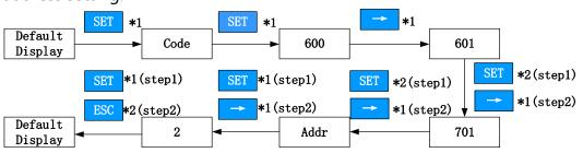
2. Meter setting for type DTSU666-3\*230V 100A/40mA and DTSU666-3\*230V 250A/50mA, three-phase meter (with CT)
