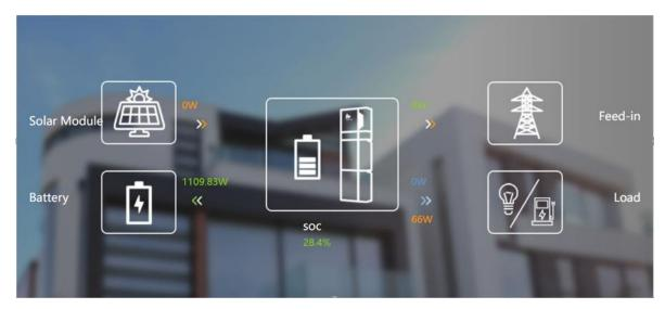
The above figure shows the real-time power map (if the system supports the latest features).
