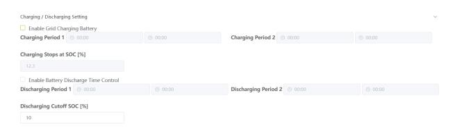
The main function of the charge and discharge setting is to set the charging and discharging time period of the system at the on-grid situation. Users should pay attention to the SOC value to prevent over charging and over discharging of the battery.
