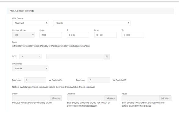
2. Select AUX 1 or AUX 2 in AUX Contact Channel. Two devices can be controlled totally.
