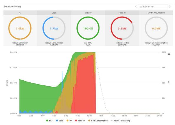
The image below shows the power diagram of the energy storage system with an EV-charger installed:
