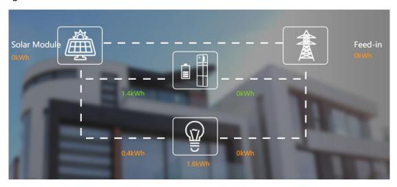
The image below shows the energy flow chart of the energy storage system with an EV-charger installed:
