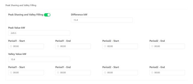
The peak-shaving and valley-filling function is only available on commercial energy storage systems, whose EMS version is above V5.03.47. The setting parameters include enable button, difference, peak value, start time and end time of peak shaving period 1, start time and end time of peak shaving period 2, valley value, start time and end time of valley filling period 2.
